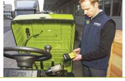
• The CLARK handset can be used for diagnostics and settings of up to 20 different performance parameters to match your requirements.
