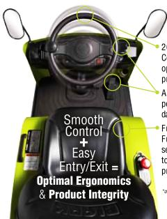
26° Tilt Steering Column maximizes operator's driving preferences.
