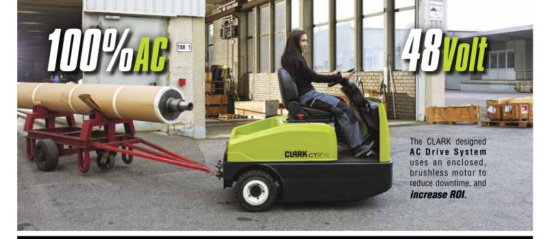
The **100% AC** 48-Volt high performance drive system, and regenerative braking, give the compact rear-wheel drive CTX exceptional **acceleration**, **speed**, and **gradeability**.
